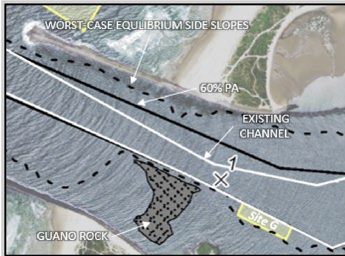
Figure 8-25: Extent of Side Slope Equilibration near Site G
