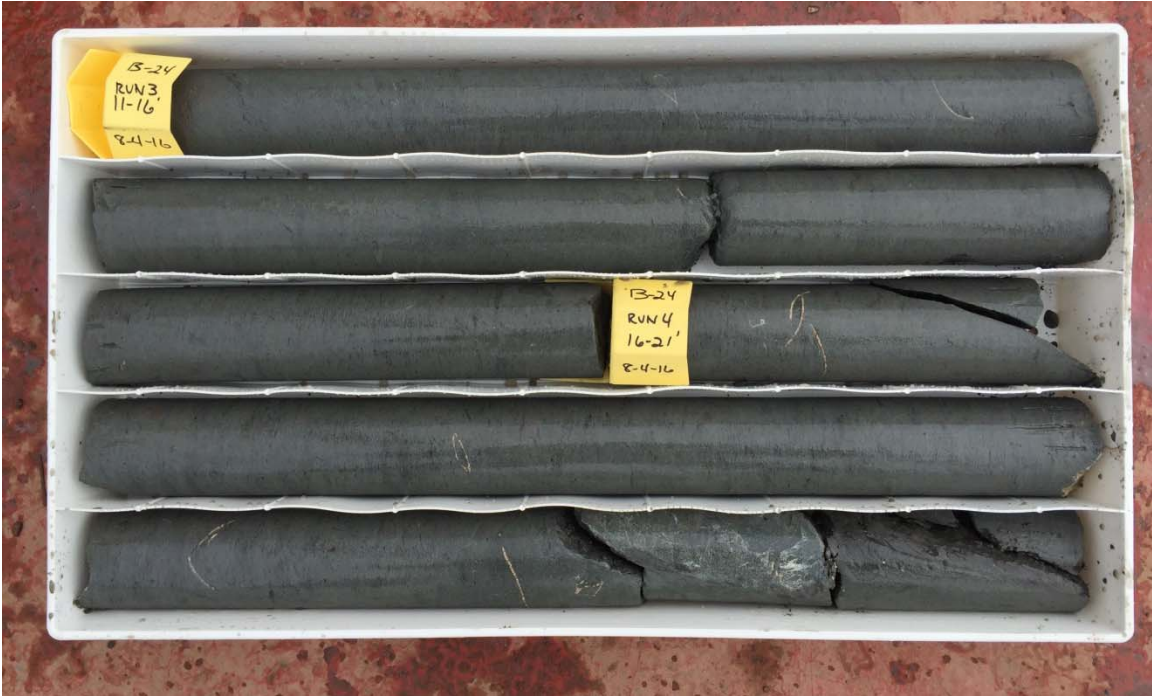
Boring 24, Run 3 to Run 4, 11 - 21 ft depth
