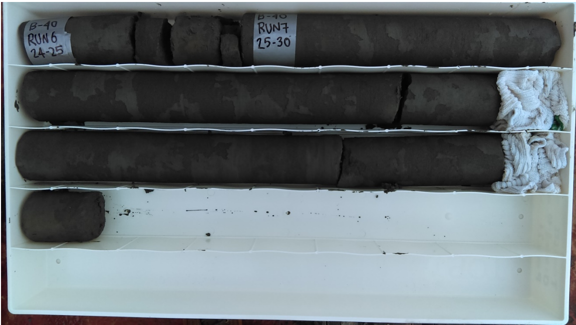
Boring 40, Run 6 to Run 7, 24 - 30 ft depth
