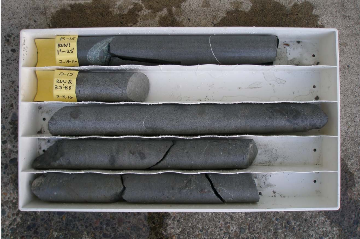
Boring 15, Run 1 to Run 2, 0 - 8.5 ft depth
