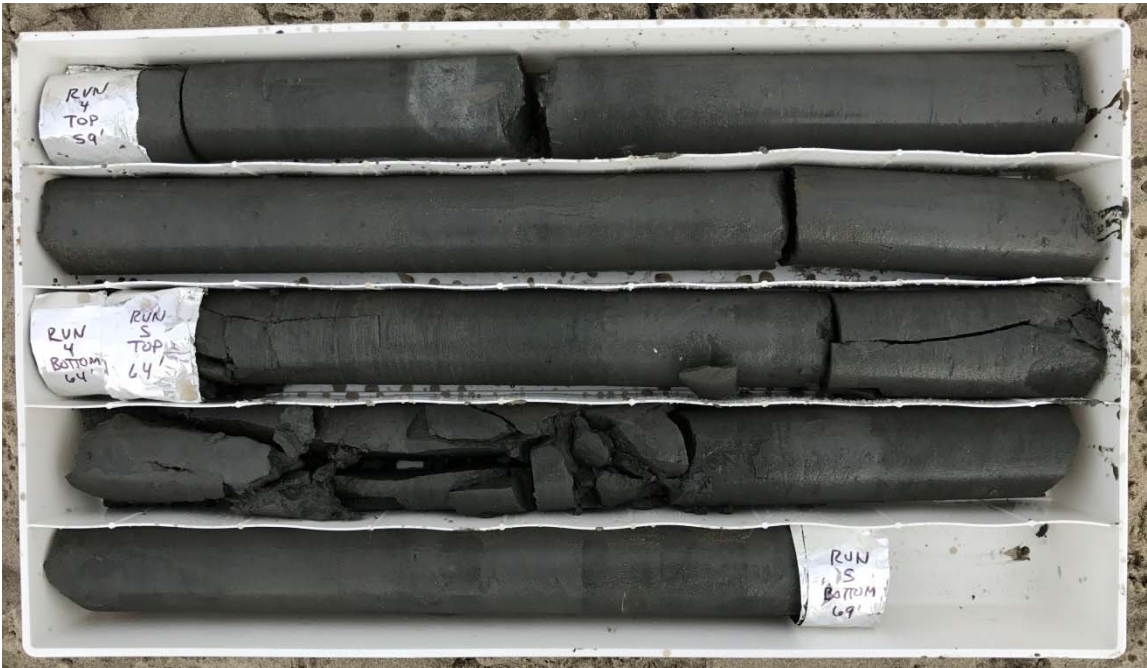
Boring UB-1, Run 4 to Run 5, 59 - 69 ft depth
