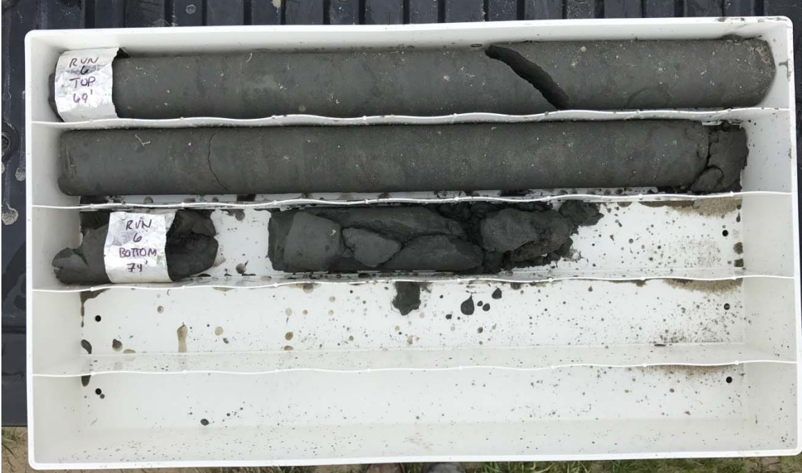
Boring UB-1, Run 6, 69 - 74 ft depth (Run 7 not photographed during field work)
