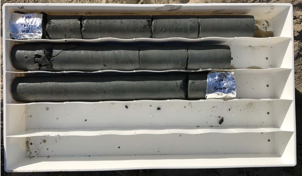
Boring UB-2, Run 5, 60 - 65 ft depth
