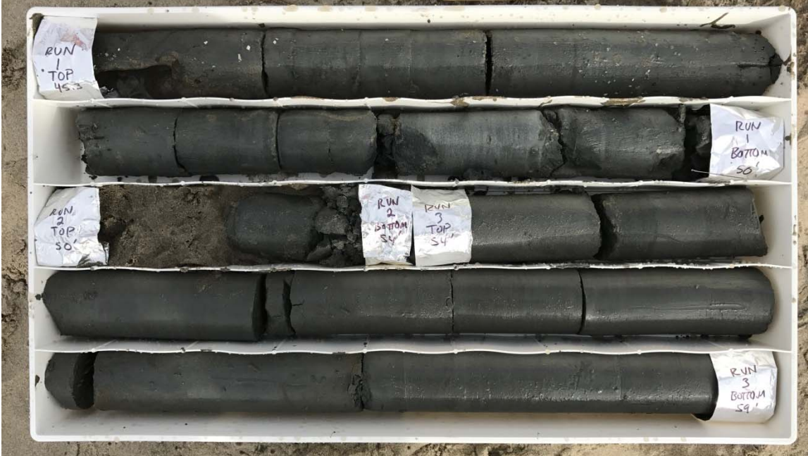
Boring UB-1, Run 1 to Run 3, 45.3 - 59 ft depth
