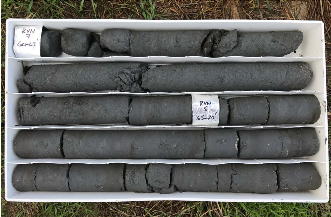
Boring UB-3, Run 7 to Run 8, 60 - 70 ft depth
