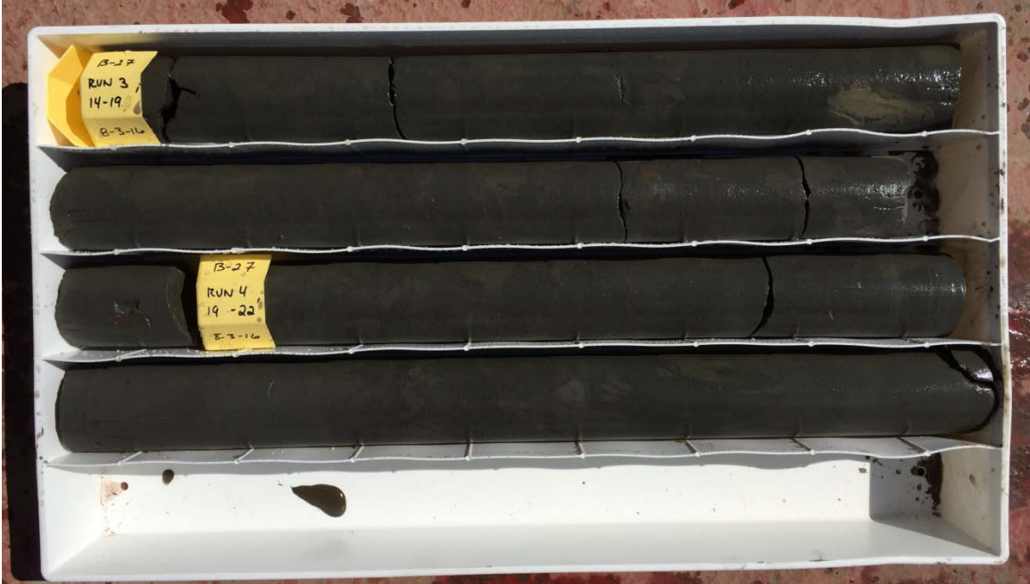
Boring 27, Run 3 to Run 4, 14 - 22 ft depth
