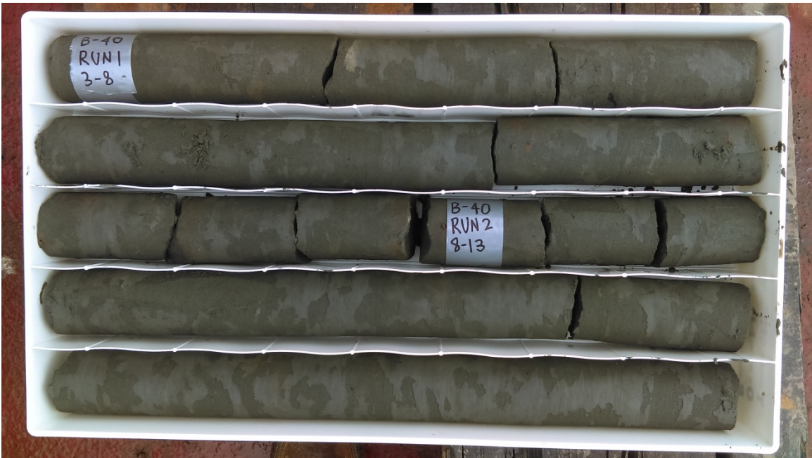
Boring 40, Run 1 to Run 2, 3 - 13 ft depth
