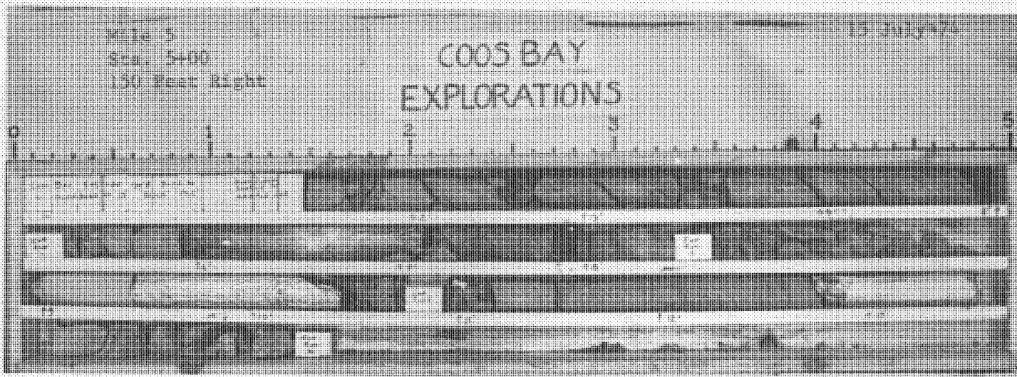
COOS BAY BORING MILE 5 STA. 5+00 150 FEET RIGHT. Sandstone . Top of rock elevation -32.1 to -33.2; Siltstone : elevation -33.2 to 39.4; Sandstone : elevation -39.4 to -41.8; Siltstone : -41.8 to bottom of hole elevation: -45.3. See Plate A-13 for log of core.
