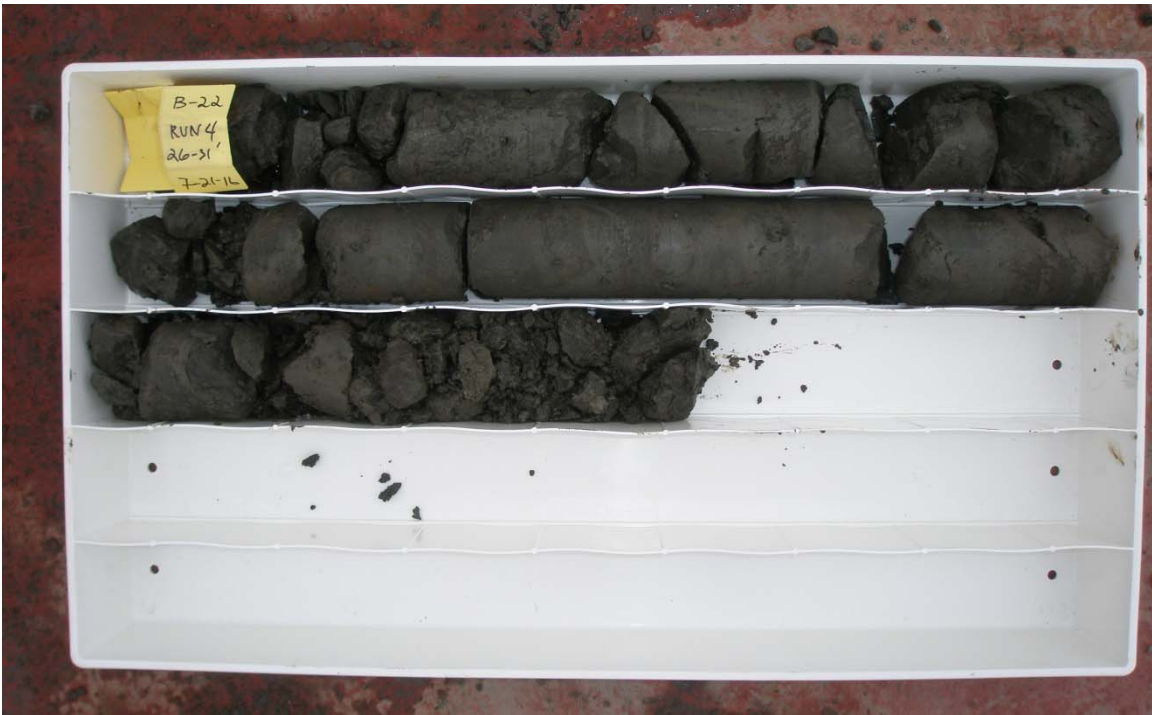
Boring 22, Run 4, 26 - 31 ft depth
