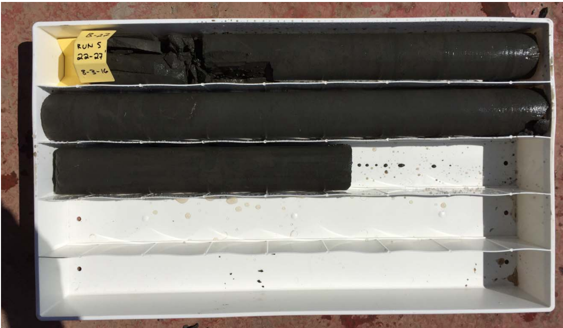
Boring 27, Run 5, 22 - 27 ft depth
