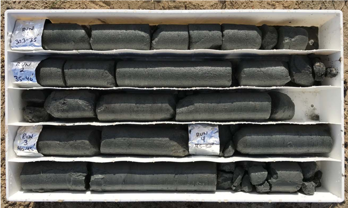
Boring UB-3, Run 1 to Run 4, 30.3 - 50 ft depth
