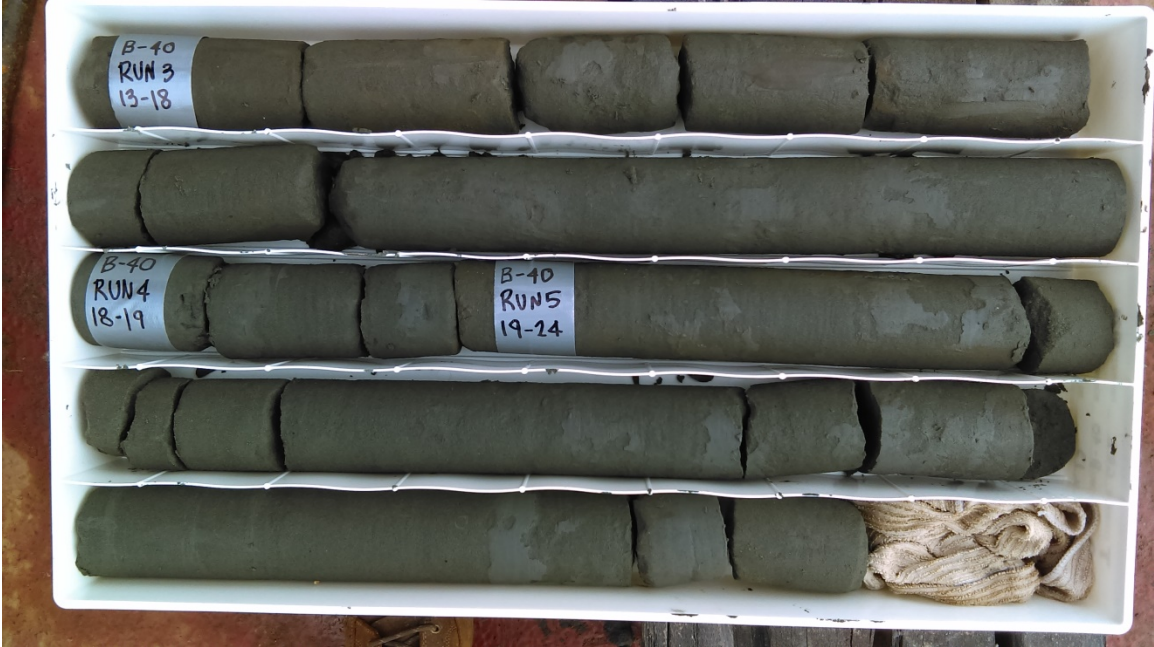
Boring 40, Run 3 to Run 5, 13 - 24 ft depth
