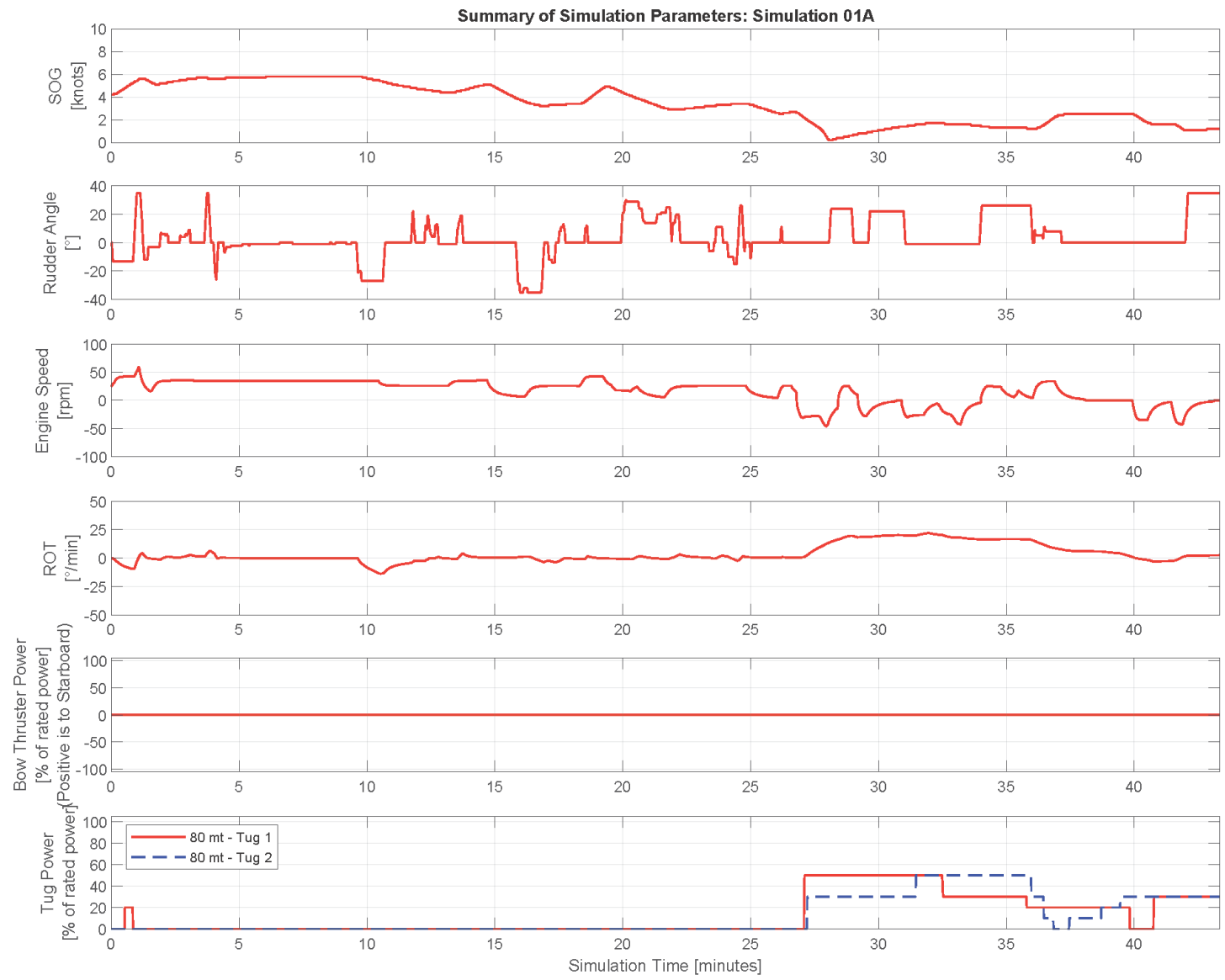
Figure 4-2. Simulation 1A Vessel and Tug Parameter Time Series
