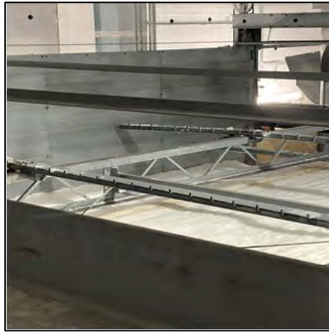
The first photo above shows a bent diagonal and rack lift beam. The second photo shows one of the ice delivery rakes that was bent from the impact of the ice chunk.
