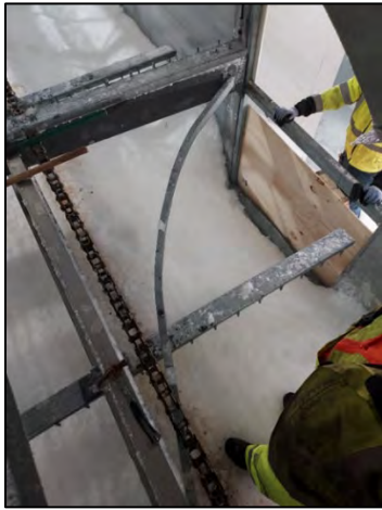
The first photo above shows a bent diagonal and rack lift beam. The second photo shows one of the ice delivery rakes that was bent from the impact of the ice chunk.
