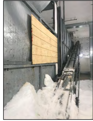
The first photo above shows a bent diagonal and rack lift beam. The second photo shows one of the ice delivery rakes that was bent from the impact of the ice chunk.
