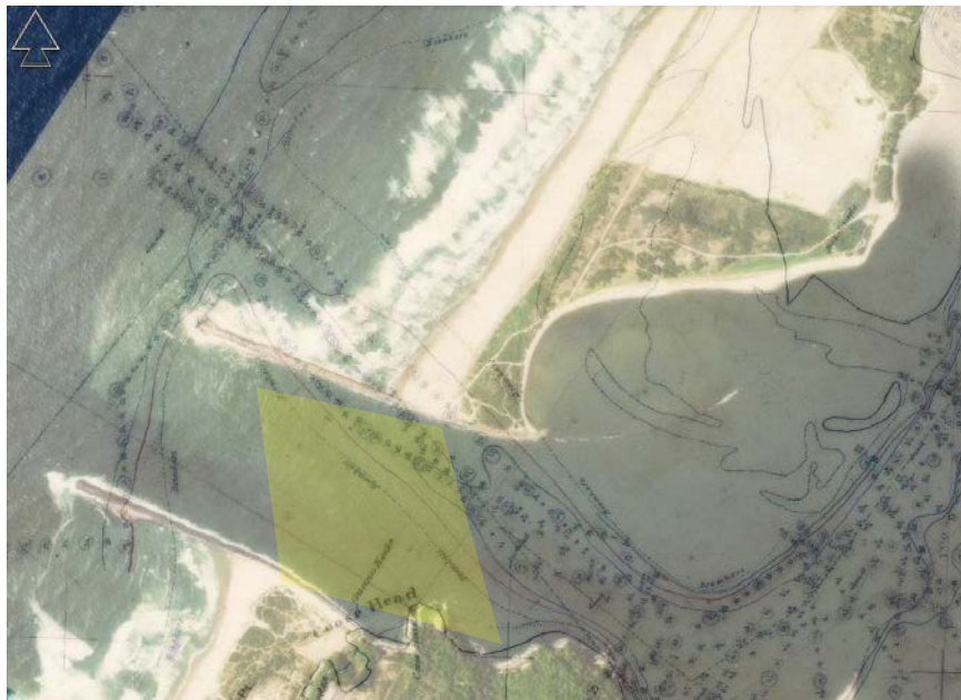
Figure 10: Overlay of the original U.S. Coast Survey (now NOAA) sounding chart of the Coos Bay Entrance channel from 1861 to a modern aerial photograph. Note the northwesterly orientation of the original river channel, possible diverted by the up-thrust area around Guano Rock (approximately yellow highlight.)
