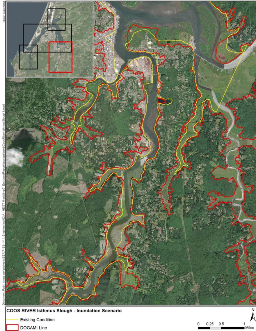
Figure 7-14 Comparison of DOGAMI XXL1 Inundation Line and MIKE-21 Existing Condition Simulation – Isthmus Slough
