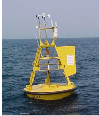
Figure 2-12 3-meter Discus NDBC Buoy
