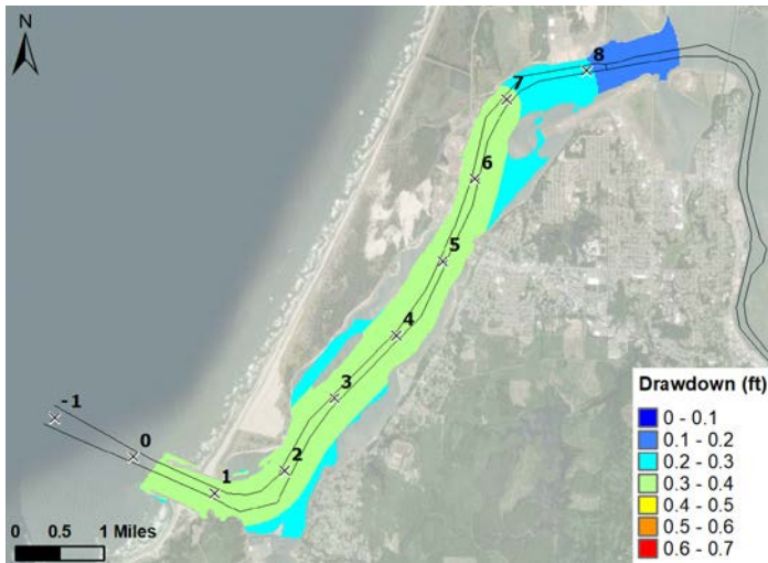
Figure 7-9 Drawdown of Case 04 - Bulk Departure, PA
