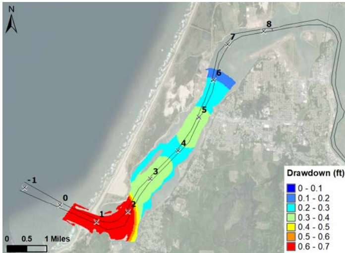
Figure 7-11 Drawdown of Case 06 - Container Ship Departure, PA
