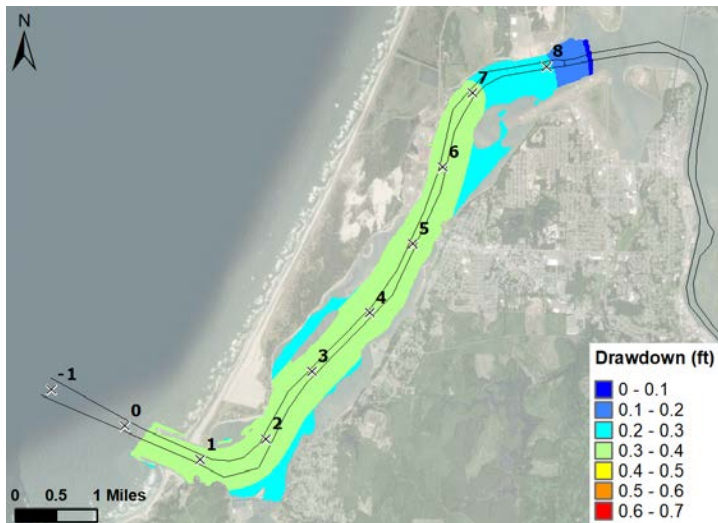
Figure 7-7 Drawdown of Case 02 - Bulk Arrival, PA
