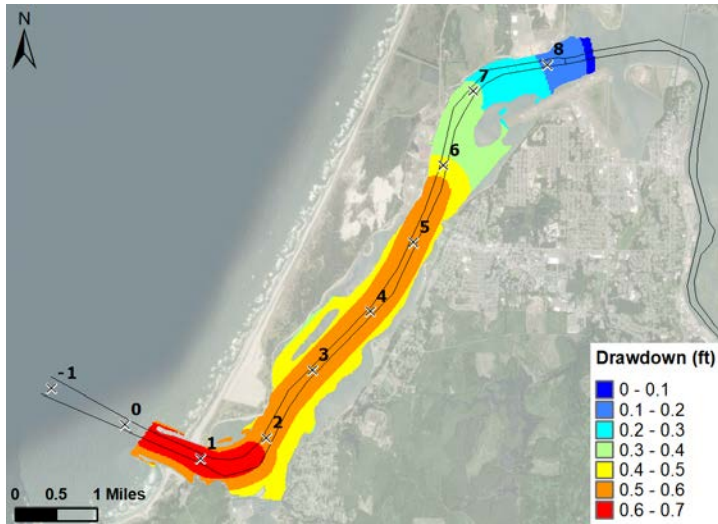
Figure 7-6 Drawdown of Case 01 - Bulk Arrival, Existing Condition
