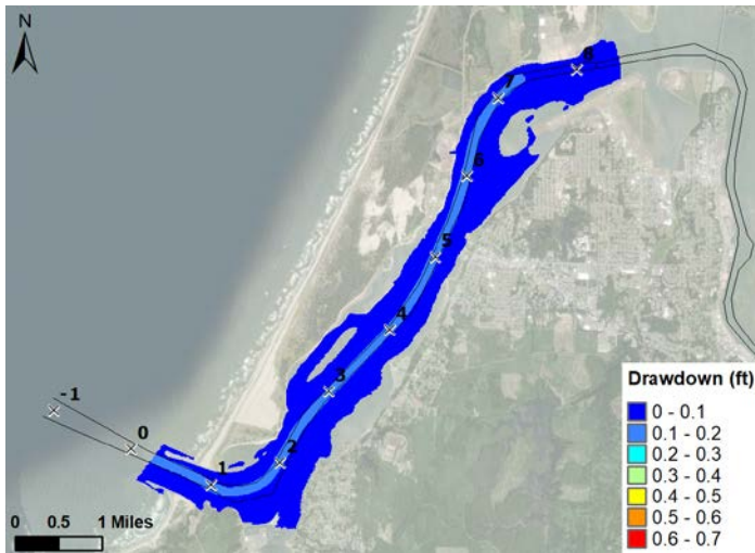
Figure 7-5 Drawdown of Case 12 – ASD Tug Departure at 12 Knots, PA
