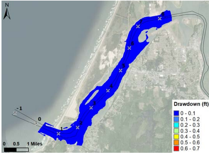
Figure 7-4 Drawdown of Case 10 – Conventional Tug Departure at 12 Knots, Existing Condition
